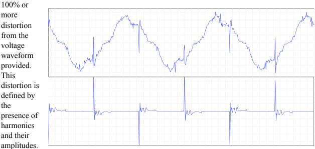
Shown above top is the applied voltage, and below it the resulting current from a nonlinear load, such as a fluorescent lamp. Note the coincidence of distortion on the voltage waveform with the pulse of current, and subsequent oscillations, on the bottom half.
